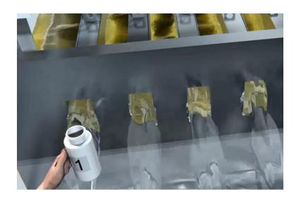
Independent monitoring and isolation of each filter element
