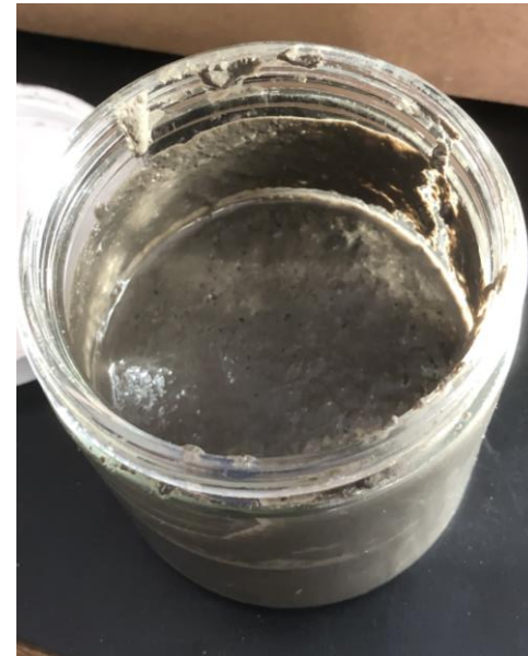
Reject Sample from Stabilized Control System, ~2% free water. Historically, observed >10% free water
