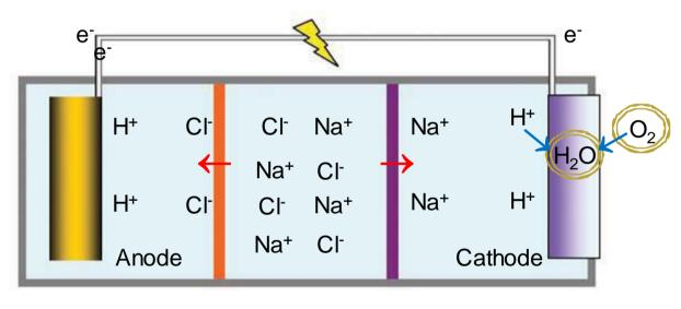
Anion Exchange Cation Exchange Membrane (AEM) Membrane (CEM)
