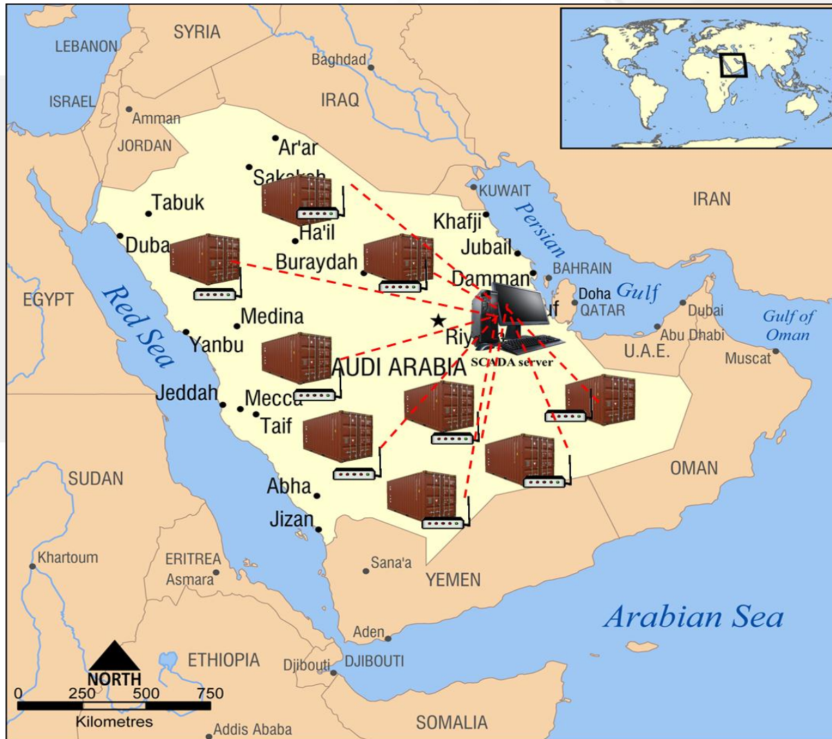
Figure 26. Illustration of SCADA implementation to control and monitoring the portable system in remote areas of Saudi Arabia
